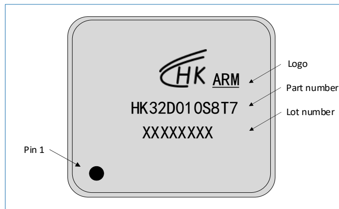
Figure 7-5 LQFP44 HK32D010S8T7 marking example
