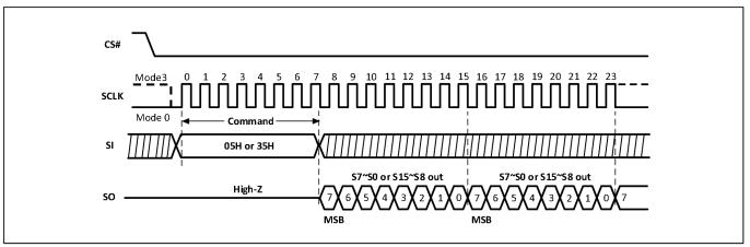
Figure-10. Read Status Register Sequence Diagram (QPI)
