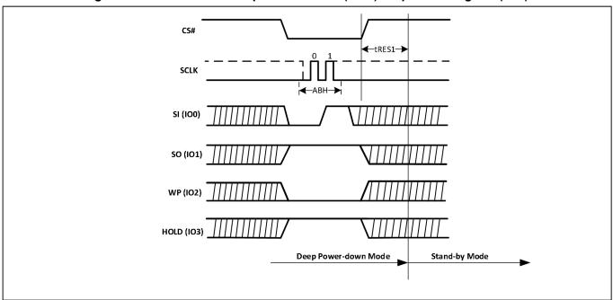
Figure-60. Read Electronic Signature (RES) Sequence Diagram
