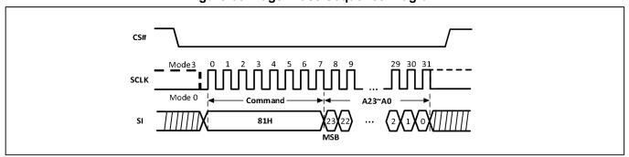
Figure-31. Page Erase Sequence Diagram (QPI)
