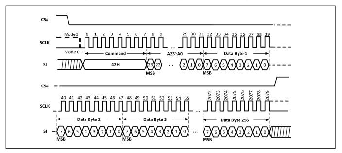
Figure-49. Program Security Register Sequence Diagram(QPI)
