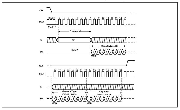
Figure-68. Read Identification Sequence Diagram (QPI)
