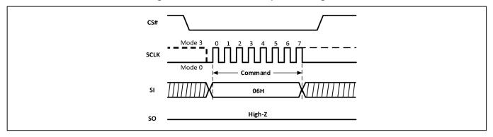
Figure-4. Write Enable (WREN) Sequence (QPI)
