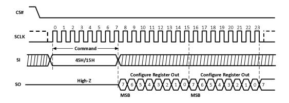
Figure-55. Read Configure Register (QPI)
