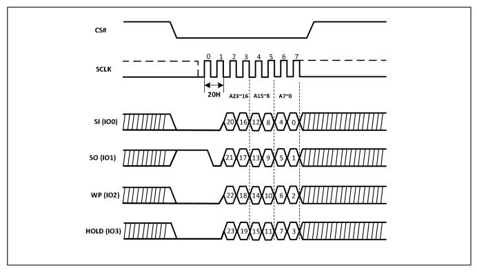
The self-timed Sector Erase Cycle time (tSE) is initiated as soon as Chip Select (CS#) goes high. The Write in progress (WIP) bit still can be check out during the Sector Erase cycle is in progress. The WIP sets 1 during the tSE timing, and sets 0 when Sector Erase Cycle is completed, and the Write Enable Latch (WEL) bit is reset. If the sector is protected by BP4, BP3, BP2, BP1, BP0 bits, the Sector Erase (SE) instruction will not be executed on the sector
