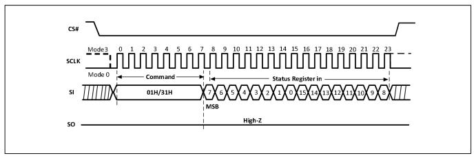
Figure-13. Write Status Register Sequence Diagram (QPI)
