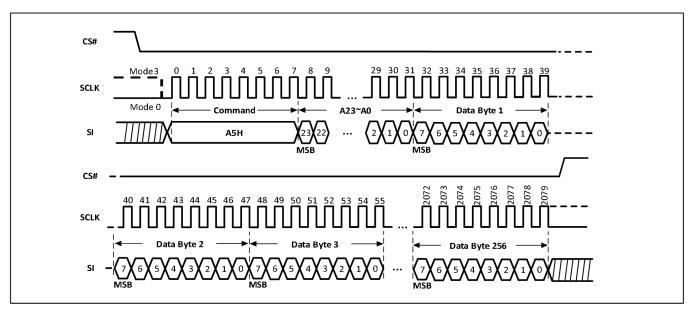
Figure-42. Page Write Sequence Diagram
