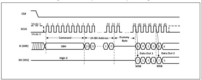
Figure-17. Dual Output Fast Read Sequence Diagram
