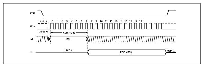
Figure-11. Active Status Interrupt Sequence Diagram
