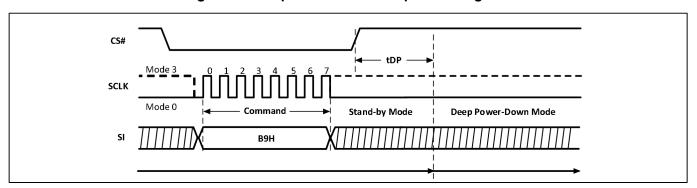
Figure-56. Deep Power-Down Sequence Diagram
