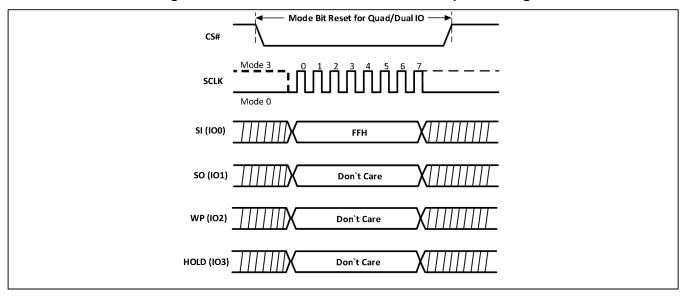
Figure-77. Continuous Read Mode Reset Sequence Diagram
