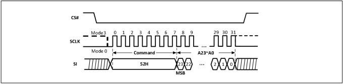
Figure-35. Half Block Erase Sequence Diagram (QPI)
