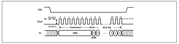
Figure-37. Block Erase Sequence Diagram (QPI)
