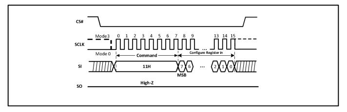
Figure 53. Write Configure Register (WRCR) Sequence (QPI)
