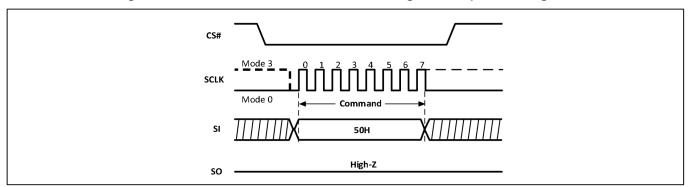
Figure-8. Write Enable for Volatile Status Register Sequence Diagram (QPI)
