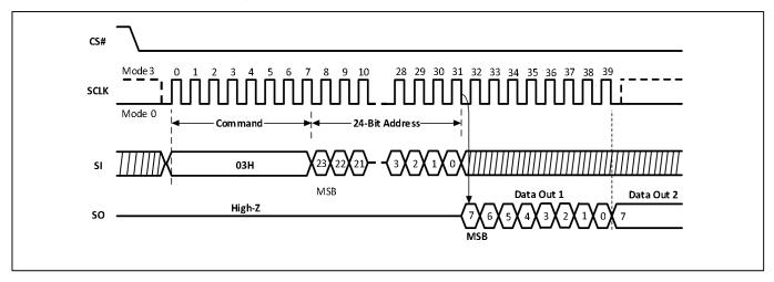
Figure-14. Read Data Bytes Sequence Diagram
