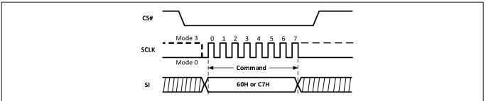
Figure-39. Chip Erase Sequence Diagram (QPI)
