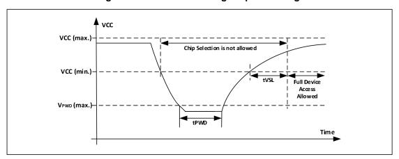
Table-14 Power-Up Timing and Write Inhibit Threshold
