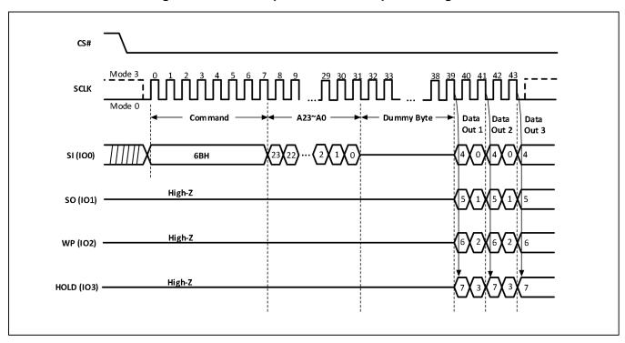
Figure-20. Quad Output Fast Read Sequence Diagram
