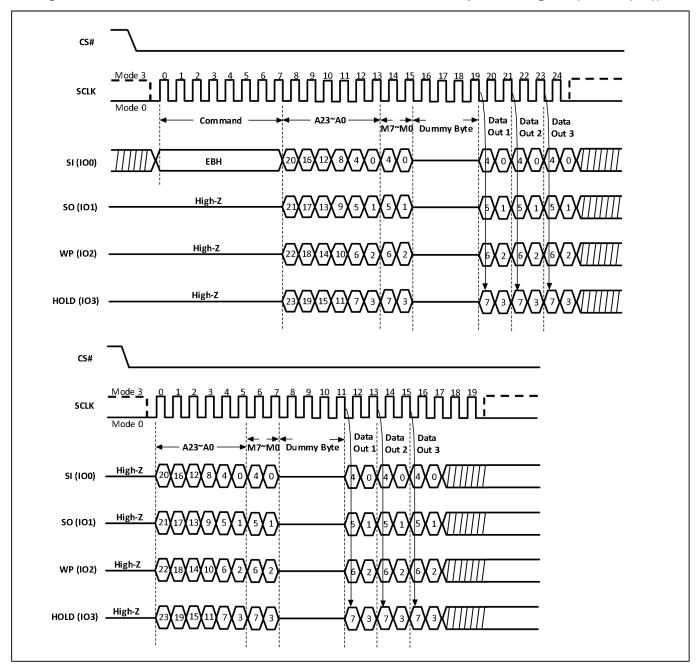
**Note**: Quad I/O Fast Read with "Continuous Read Mode", if (M5-4)=(1,0). If not using "Continuous Read Mode" recommend setting (M5-4)≠(1,0).
