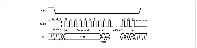
Figure-47. Erase Security Register Sequence Diagram (QPI)
