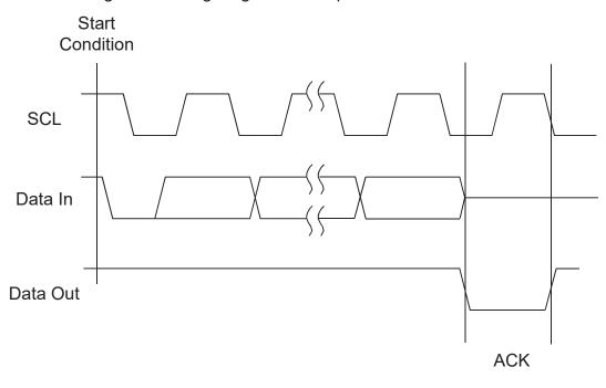
Figure 2: Timing diagram for output ACKNOWLEDGE
