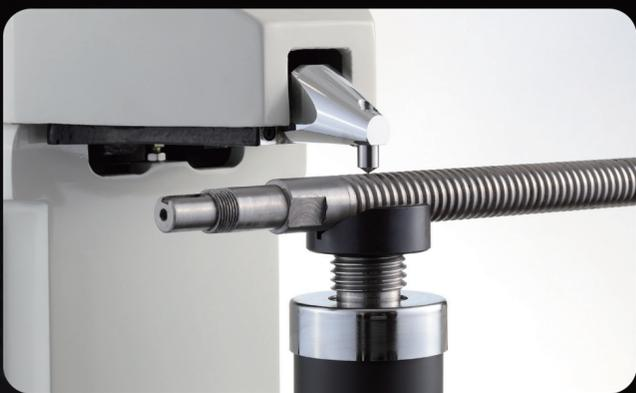
**NO.5** Screw lead hardness test
