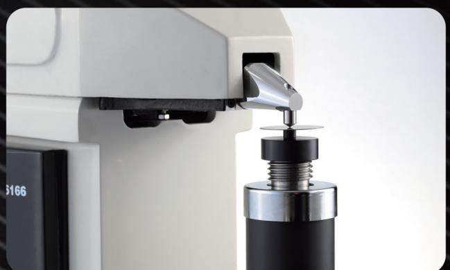
**NO.8** Use diamond specimen support to test HR30Tsm and HR15Tsm of thin tin plate
