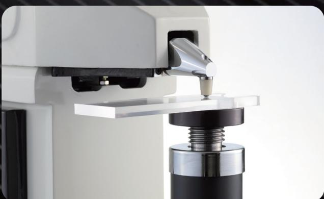
**NO.7** Plexiglass plate plastic Rockwell HRMW test
