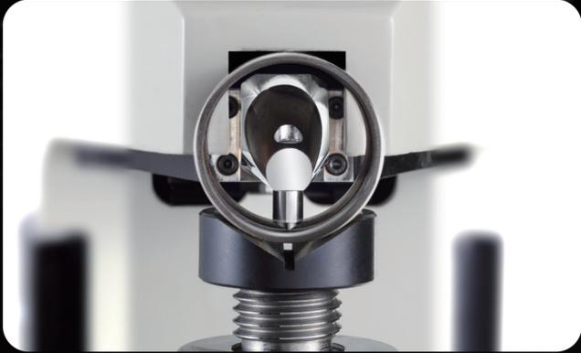
**NO.1** Ring/pipe inner wall hardness test
