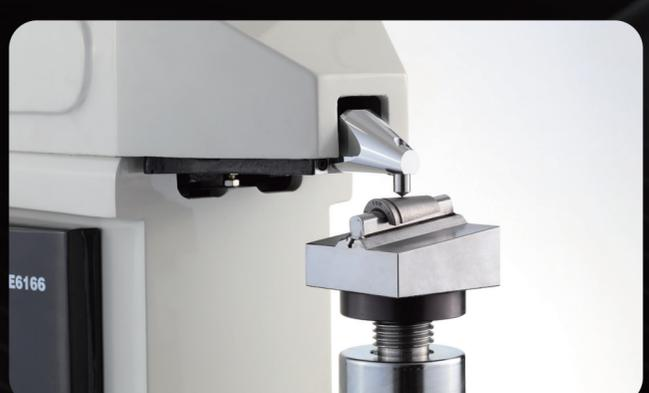
**NO.6** Hardness test of anchor clip
