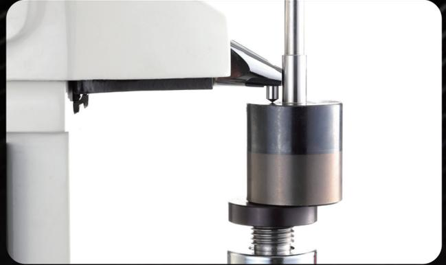
**NO.2** Stepped sample hardness test
