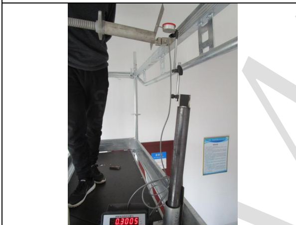
Fig.7 Elastic deflection of side protection during the horizontal loading
