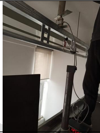
Fig.6 Elastic deflection of side protection during the downward loading
