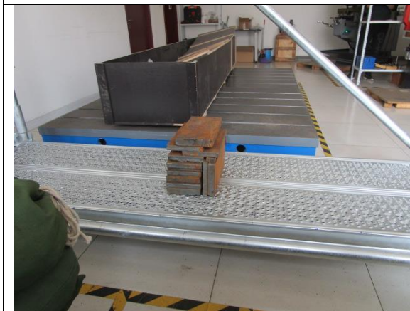
Fig.3 Working area during the concentrated load over an area of 200mmx200mm
