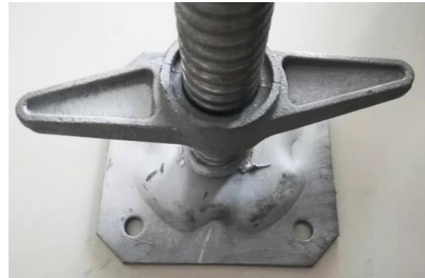
Fig.10 Scaffold base after test
