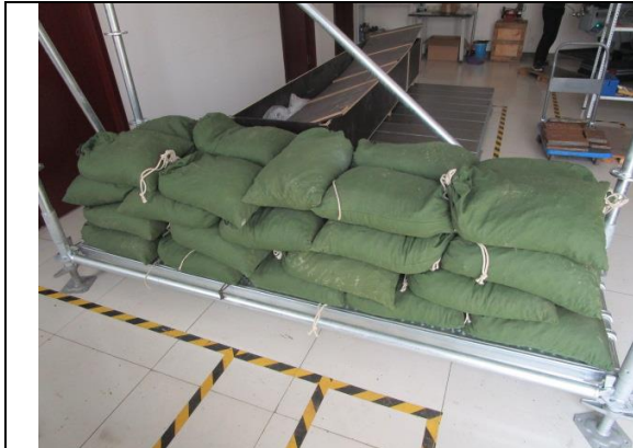
Fig.1 Working area during the uniformly distributed service load
