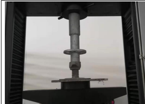
Fig.9 Scaffold base during test
