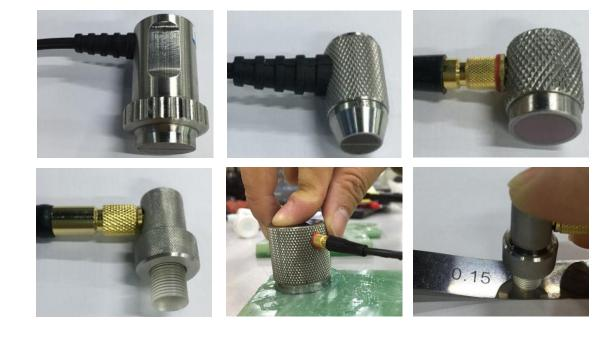
The standard echo detection mode measures the thickness based on the time interval between the excitation pulse and the first back-wall echo. User can measure uncoated materials in this mode.
